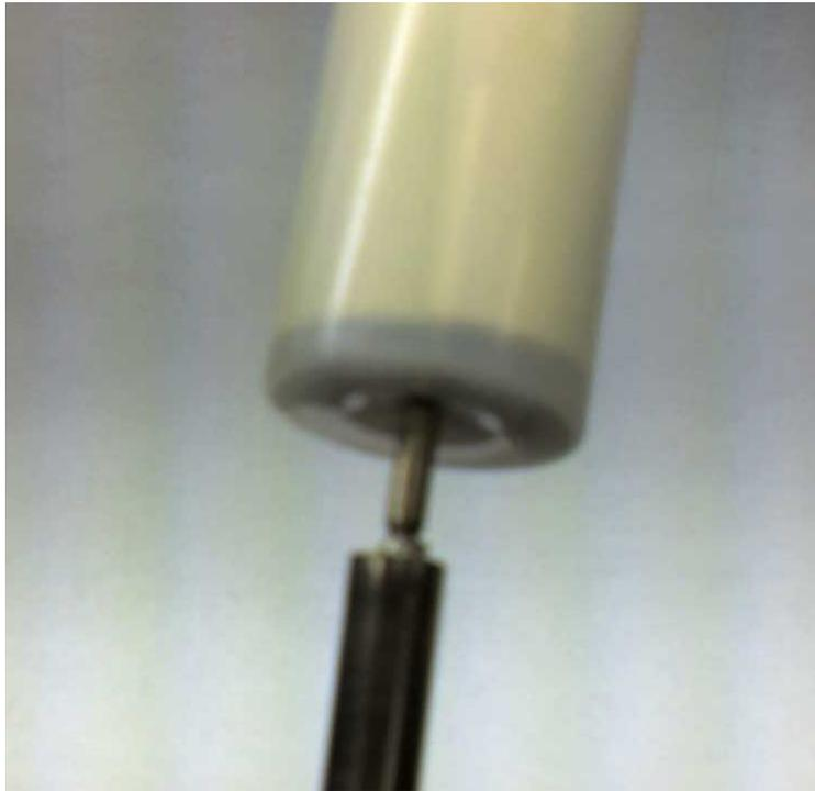
6. Once the motor is in keep the assembly in the iron for a good 5 seconds then slide the motor/coupler assembly out of the iron. You may need to use pliers to help if the tinfoil is too tight.
