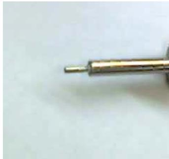
4. Its now time to warm up the iron. Once the iron is hot, place a coupler into the tinfoil (which should already be in the iron). Once the coupler starts to get warm place the solder down the throat of the cup. As it starts to melt, GO SLOW!!! Let the Flux bubble out a bit.
