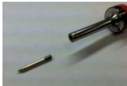
2. Now we have a nice hole in the end of our iron, if your real lucky the coupler fits right in the end threads first and stops when the body of the coupler gets to the iron. You can use the set screw to assist this if are close, otherwise fear not, that's what the tinfoil is for!
