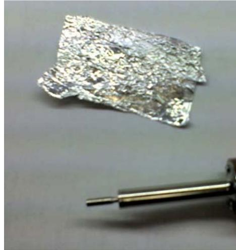
3. Wrap the tinfoil around the coupler loosely until it is snug in the hole in the end of the iron. Wiggle the coupler around to make enough room for the coupler to come out of the foil easily.
